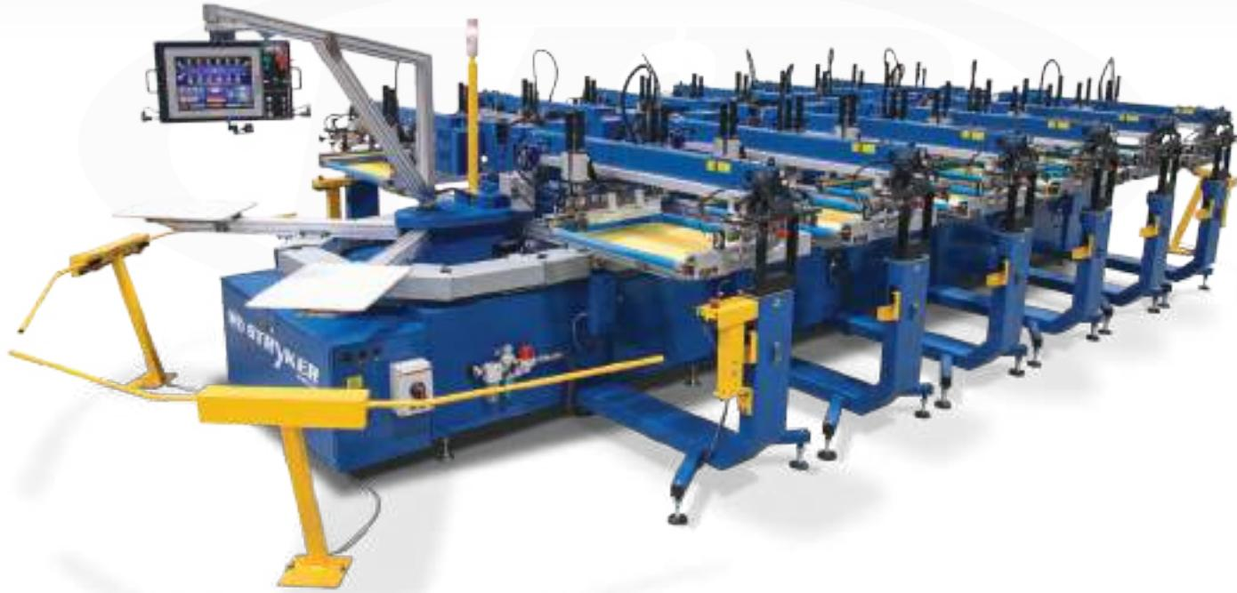
M&R's Stryker sets the standard for oval format screen printing presses. Its oval design takes up less floor space than comparable carousel automatic screen printing presses, making more efficient use of the available production area. Available in three print format sizes and expandable from 10 to 52 stations with selectable printhead locations, the Stryker can be tailored to almost any production requirement, floor layout or shop size.
